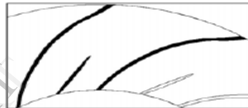
Figure 6. splitter vanes at mid span of leading edge
