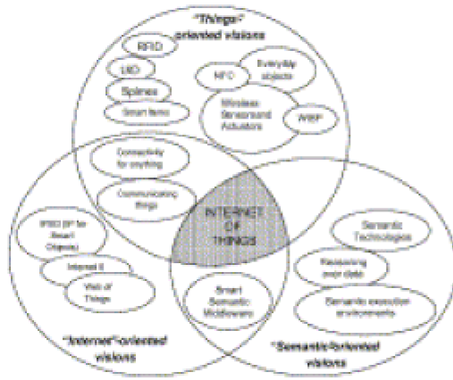
Fig 2: "Internet of Things" paradigm as a result of the convergence of different visions.
