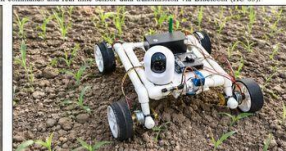
Fig. 6. Experimental setup in agricultural environment for real-time monitoring intrusion detection.
