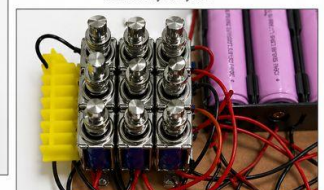
Fig. 5. Solenoid-Based Braille Actuation Mechanism
