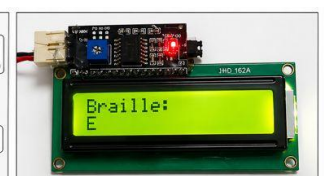
Fig. 4. LCD Display Showing Braille Output Generated by the System
