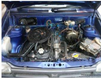
Fig:4 vaporizer fitting arrangement engine
