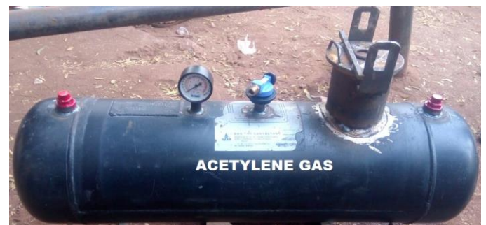
Fig:2 Acetylene gas tank
