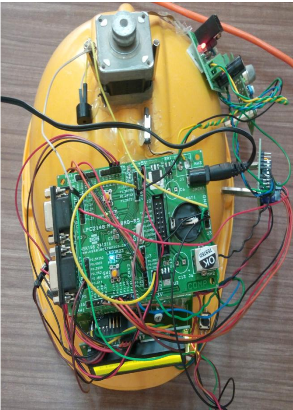
Fig 9: An Intelligent ultrasonic helmet system for Miner
