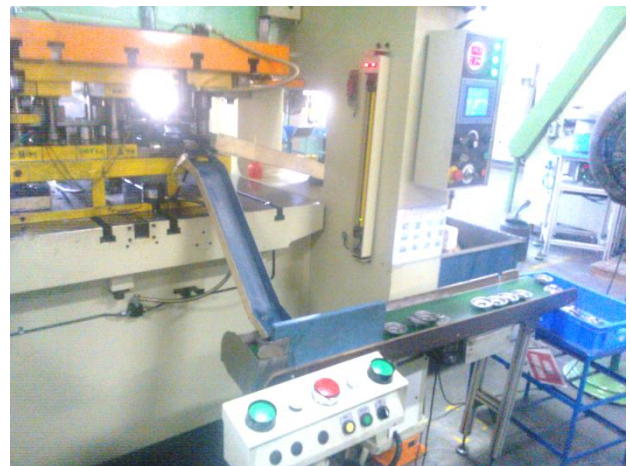
Fig 2.1 Semi-finished part collection with bin
