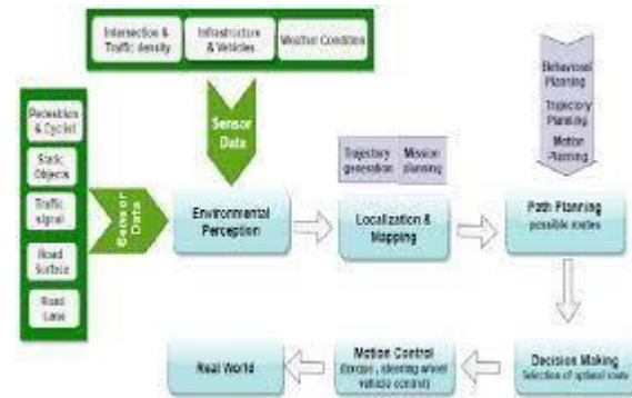
Figure 2: Workflow of the proposed deep learning-based autonomous driving system
