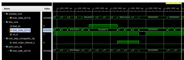
Fig. 5. Simulation waveform of delayed lockstep execution with a fault injected into the main core and the resulting comparator alert.
