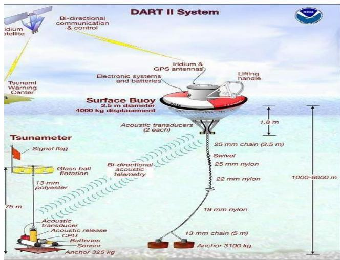
*Schematic of a NOAA DART II Buoy Station. Each DART station consists of a bottom pressure sensor ("Tsunameter") anchored to the seafloor and a companion, moored surface buoy. An acoustic link transmits data from rock bottom pressure sensor to the surface buoy, then satellite links relay the info to NOAA tsunami warning centers, giving NOAA forecasters real-time data about tsunamis that would potentially impact coastal areas. Courtesy of NOAA.[1]*
