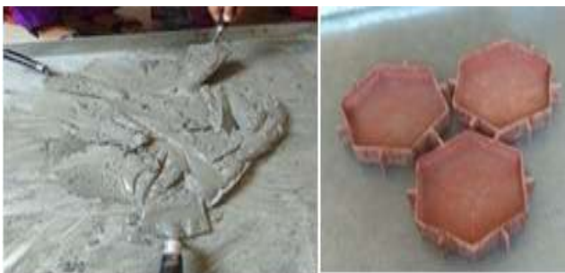
Fig. 2. Mixing and Mould for Paver Blocks
