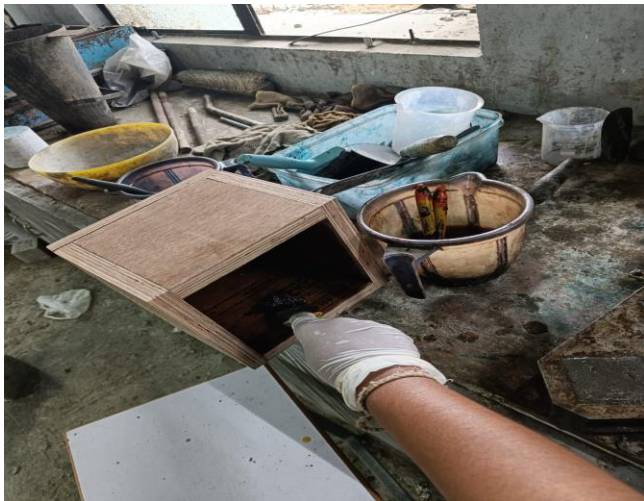
Fig 7: Greasing the mould.
