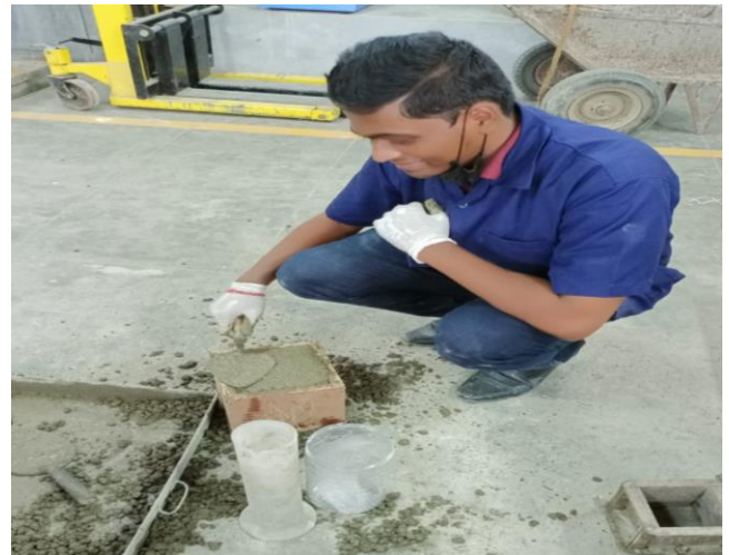
Fig 10: Finishing the concrete surface
