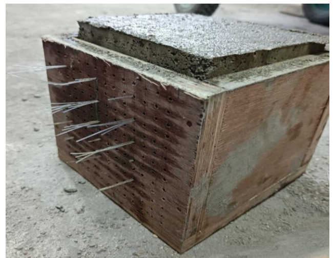
Fig 11: Demoulding the concrete
