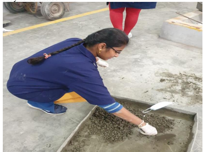
Fig 6: Wet mixing of concrete
