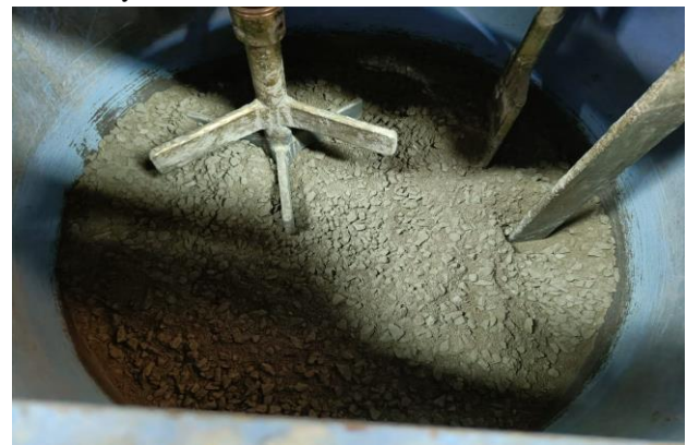
Fig 5 : Dry mixing of concrete
