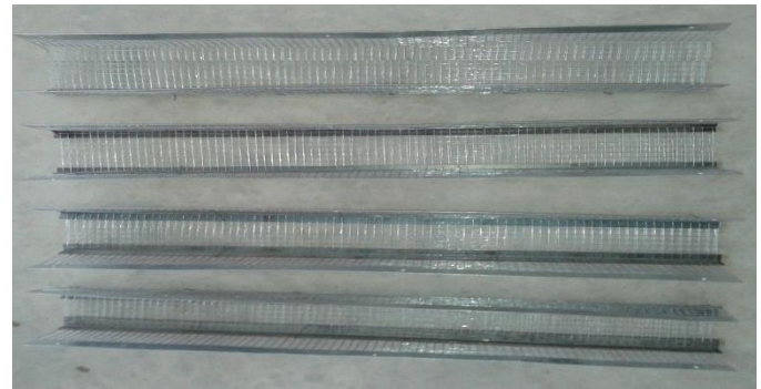
Fig.5 Expanded galvanized steel wire mesh with and without two longitudinal steel angles 10x10x3 mm, 20x20x3 mm and 30x30x3 mm
