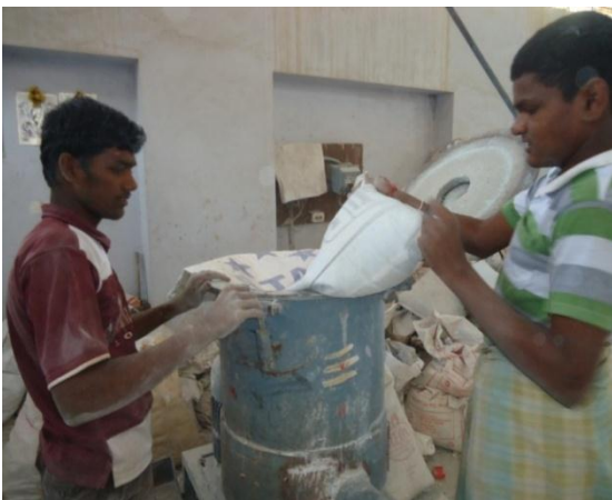
Fig(3) Step 3 – Crushed plastics-putting into grindingM/C
