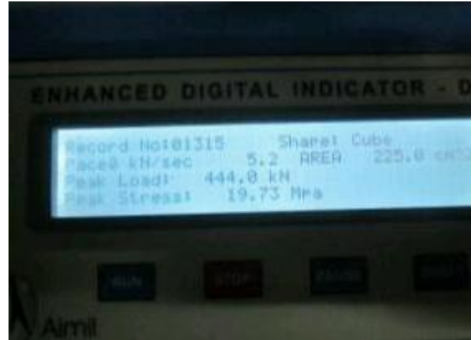
Fig (8) Test result observation in CTM machine
