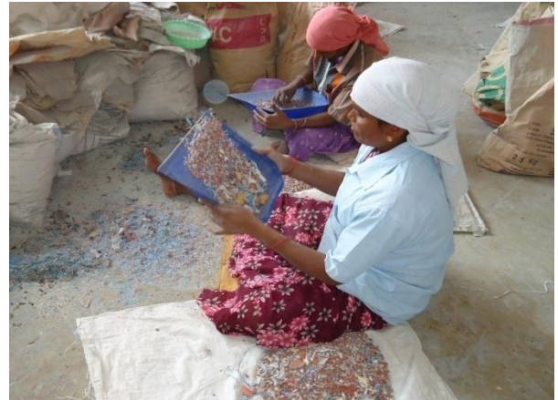
Fig(4) Step 4 – Dust removal from grinded plastics
