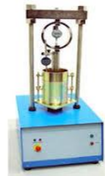
Figure 5: California Bearing Ratio Testing Machine
