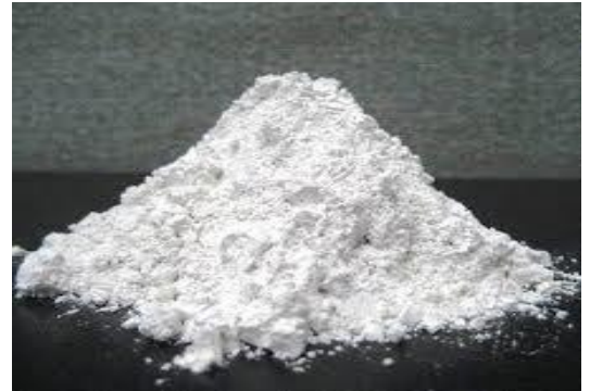
Figure 2 : Lime used in the experiment along with fly ash as a stabilizing Agent .
