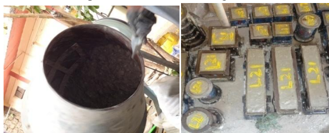
Fig 1: Mixing of concrete and concrete placed in moulds
