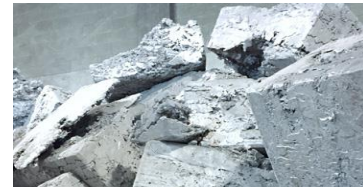
Fig.1: White dross in lumps form with high aluminium content
