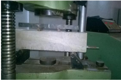
Flexural Strength Test Arrangement
