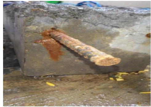
Corroded Rebar Due to the Accelerated Corrosion Technique.
