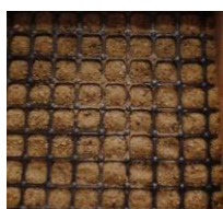
Picture-3.1: Geogrid Used In This Study
