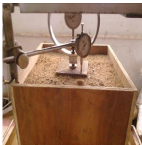
Picture 4.4: Setup of Square Footing
