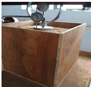
Picture 4.5: Setup of Circular Footing
