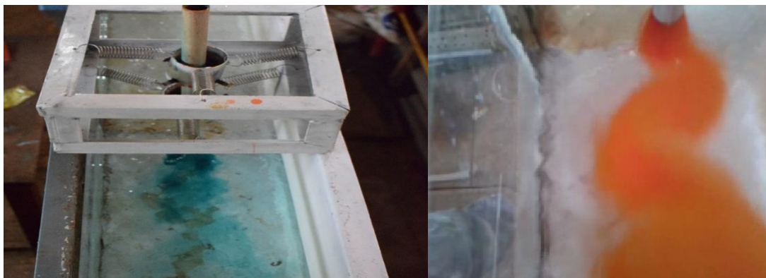
Fig:2 visualization of vortex shedding
