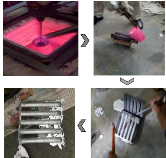
Fig 3. Stir casting and moulding process
