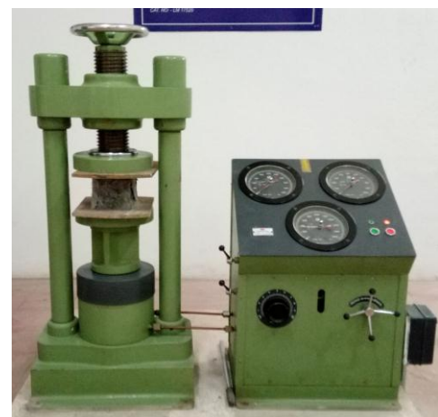
Fig 4: Compressive strength testing
