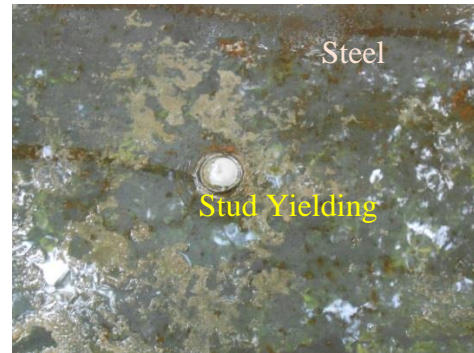
Fig.4: Stud yielding in steel
