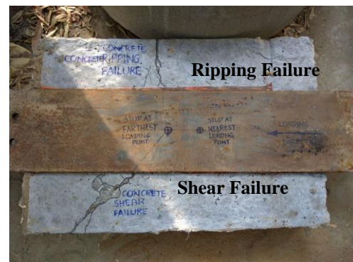
Fig.6: Ripping and shear failure in concrete
