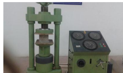
Fig1: Cubes Testing In Compression Testing Machine
