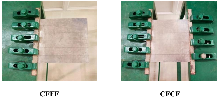
Fig 6. Five layered FML square plate (Ti/GF-E/GF-E/GF-E/Ti) under CFFF, CFCF plate boundary scenario
