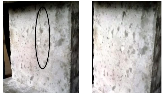
Fig.5 Crack healed concrete specimen With crack (left) & Healed Specimen (right)
