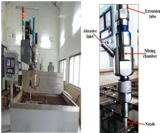
Fig. 3. Experimental set up for machining of banana FRP composite and nozzle assembly
