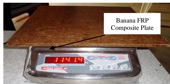
Fig. 2. Banana fiber reinforced composite plate prepared from banana fiber and unsaturated polyester resin
