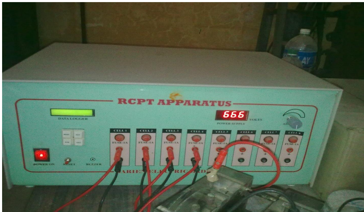
Fig: 3 Experimental Set Up Of Rcpt Test
