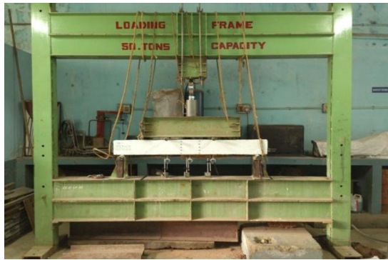
Fig. 4 Test set-up under loading frame
