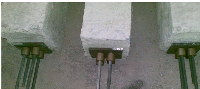
Fig. 1 Wires with end plates, barrel and wedge.
