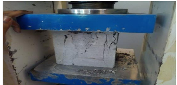
Fig 2: Testing of Concrete cubes
