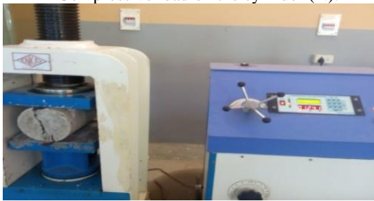
Fig 3: Testing of Cylinders
