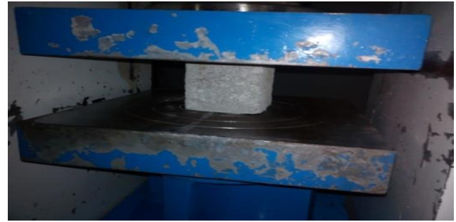
Fig 1: Testing of Mortar cubes
