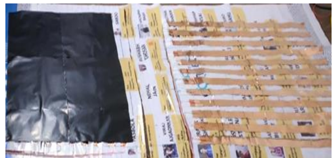
Fig 4. Velostat placed between copper strips for back mat
