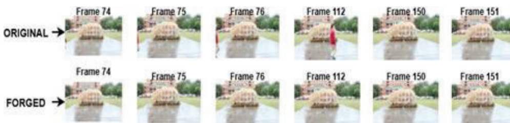
Fig.4 Original and Forged Frame Sequences for Frame Deletion case example
