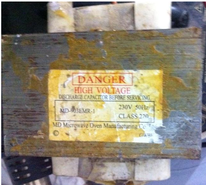
Figure 2: High voltage Step-up transformer
