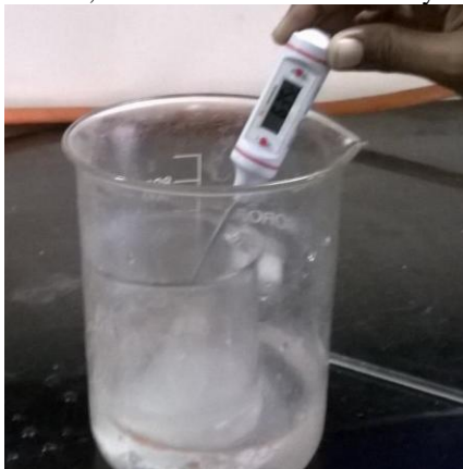
Fig. 1. Reaction of Phosphorous pent-oxide with water in presence of calcium oxide
