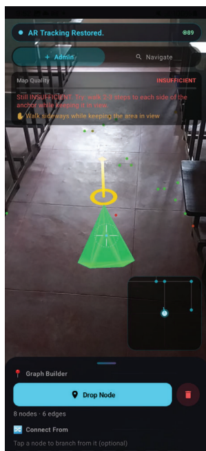
Fig. 2: Real-time AR-based indoor navigation interface showing tracking status, device position, path visualization, and destination nodes.
