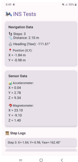
Fig. 1: Real-time IMU sensor data visualization interface
