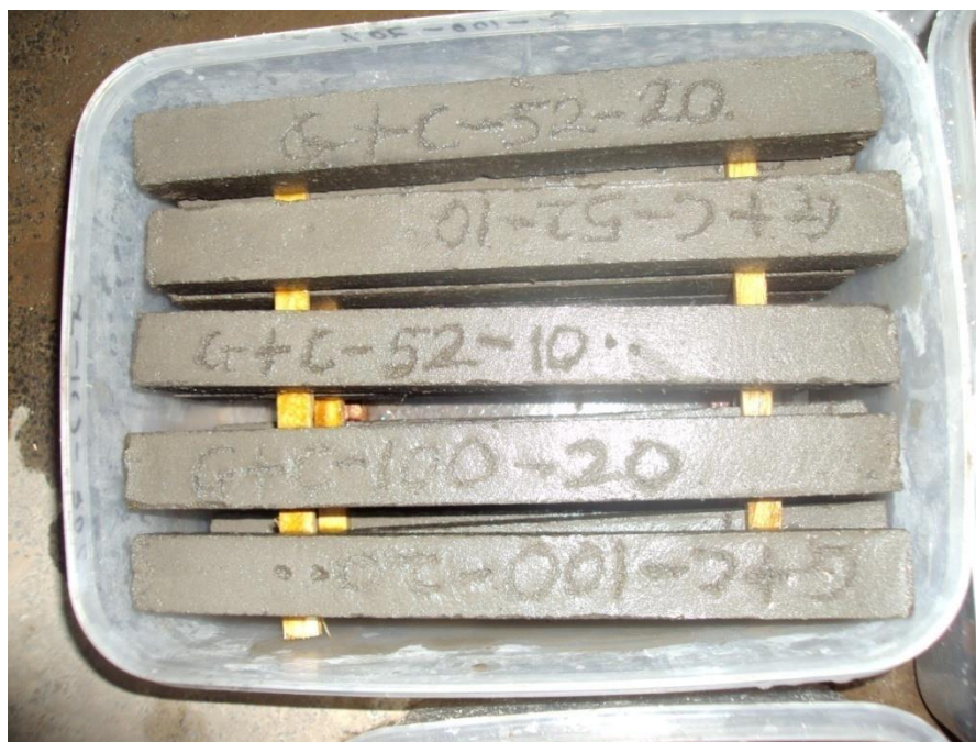
Plate 3: mortar bars placed in plastic containers ready for curing
