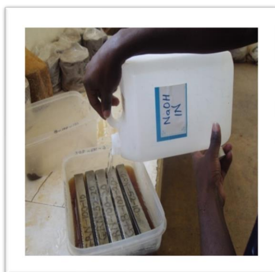
Plate 4: Addition of sodium hydroxide{1N} and Distilled Water.
