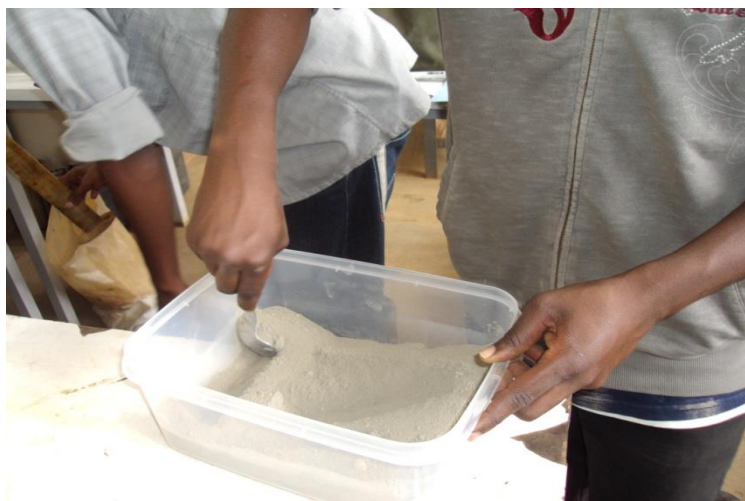
Plate 3.3h: Dry mixing of the measured quantities
