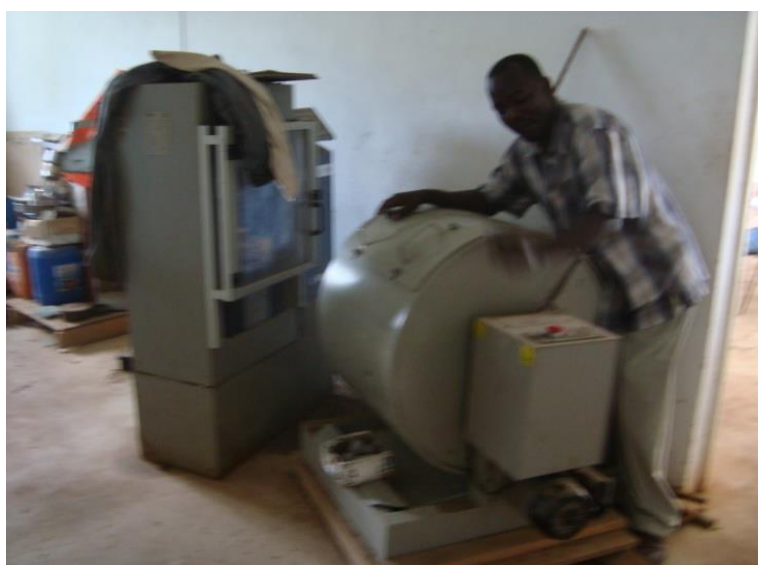
Plate 3.1.2k: Los Angeles Abrasion equipment
