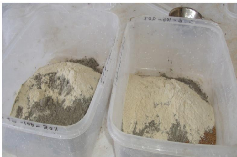
Plate 3.3g: weight quantities of cement, sand and glass ready for mixing
