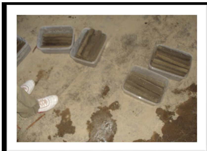
Plate 1:mortar bars placed in plastic containers after stripping / demoulding
