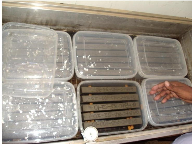
Plate 6:curing process with temperature maintained at 80°C
