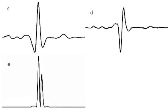
Figure 05: The process of transformation of the ECG waves, a-wave input, b-after the LPF noise reduction, noise reduction with HPF c-, d-vertices Q, R, S have been made more prominent, e-amplification peaks Q, R, S and eliminate other points.
