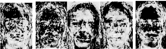
Figure 4: The Eigen Faces for the set of input facial Images (PCA Approach)
