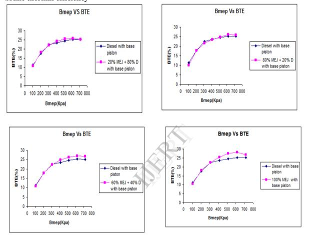
**The definition of BMEP Is:** the average (mean) pressure which, if imposed on the pistons uniformly from the top to the bottom of each power stroke, would produce the measured (brake) power output.
