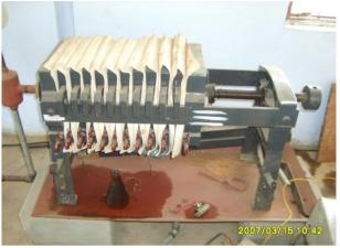
The crushed oil is then passed through a tube to the filtering chamber and thus the oil is purified to an extent.
