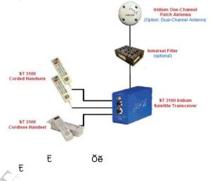
For optimum operation with Aircell Swift broadband, aircell offers a complementary Inmarsat Filter.
