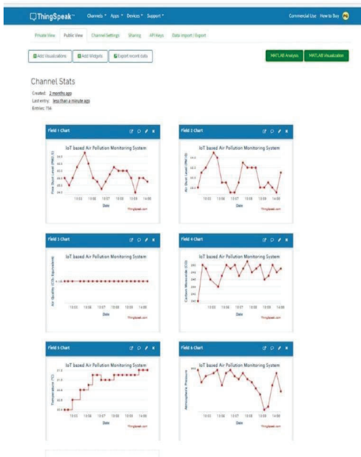
FIG. 3. REAL-TIME SENSOR DATA VISUALIZATION ON THINGSPEAK CLOUD PLATFORM
