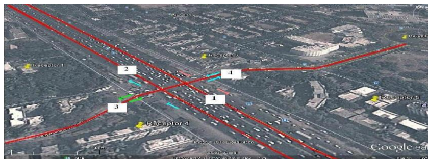
Fig. 1 Schematic of the Kherwadi intersection, Mumbai; 1 = Andheri to Mahim, 2 = Mahim to Andheri, 3 = Ram Mandir Road, 4 = S D Road
