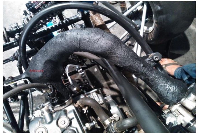
Figure 16 Top View of Intake System Assembly
