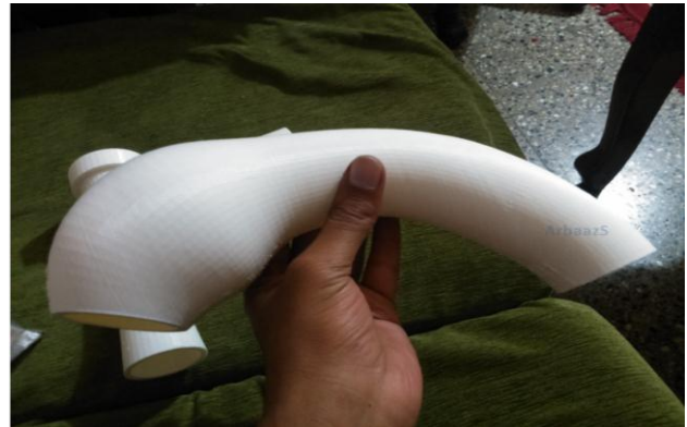
Figure 12 Rapid Prototyped Plenum
