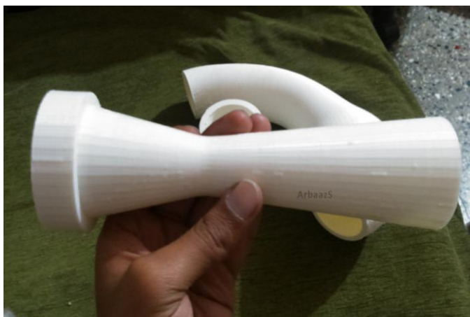
Figure 11 Rapid Prototyped Venturi
