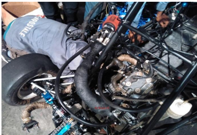
Figure 15 Intake system assembled on FSAE car
