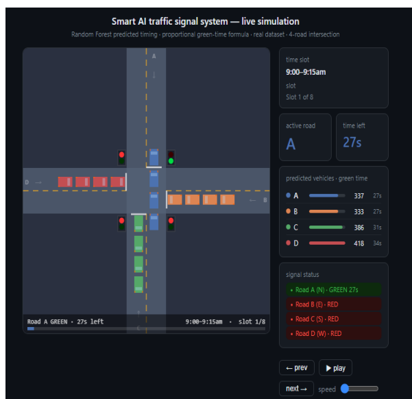
Fig. 4. Live Simulation Screenshot — AI-Based Smart Traffic Signal System
