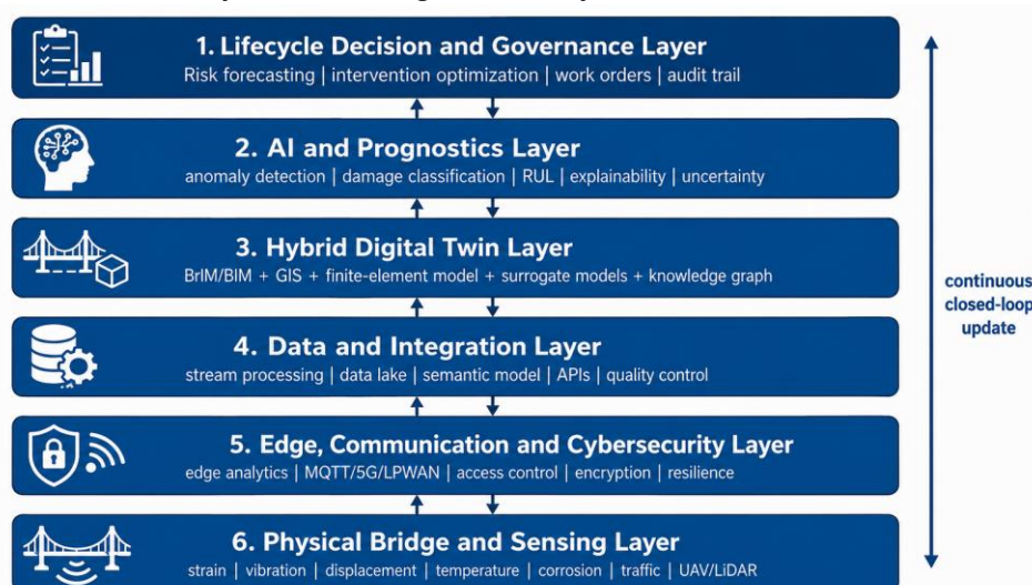
Figure 1. Layered architecture of the proposed AI-driven digital twin for bridge lifecycle management.
