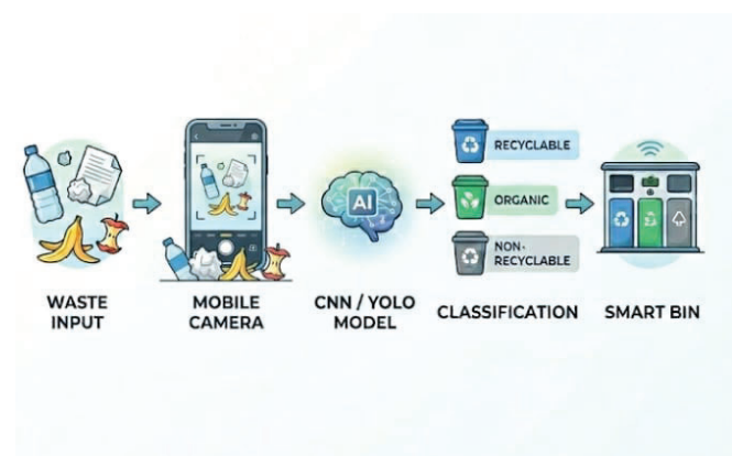
Fig. 1: AI-based waste classification pipeline from image capture to smart bin segregation
