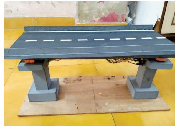
Figure 3.1 shows the fabricated bridge prototype used for experimental validation.
