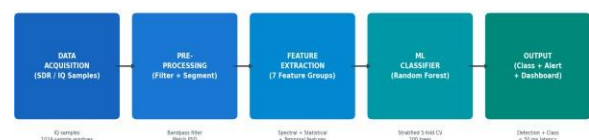
Fig. 1. Proposed end-to-end RFI detection and classification pipeline.
