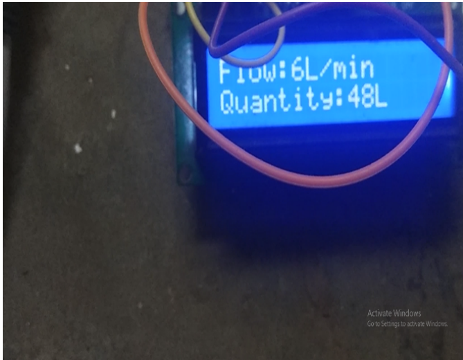
Fig. 5. LCD depicting flow rate and quantity of water discharged into field.
