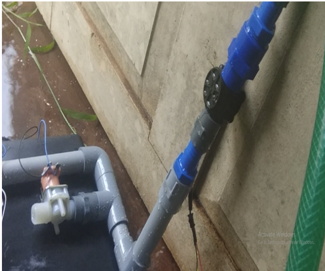
Fig. 4. Flow sensor interfaced at the junction.
