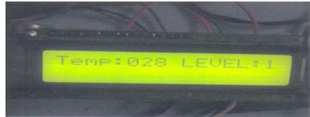
Fig7: Indication of water level 1
